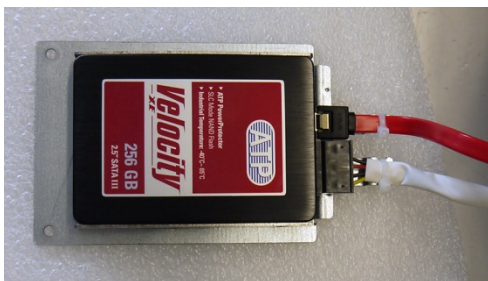
Figure 13: 2.5" Harddisk with power (white colour) and data cabling (red colour)
